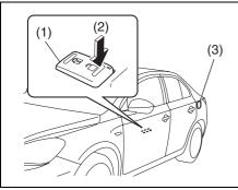
The fuel filler door (3) is located on the left rear side of the vehicle. To access the fuel filler cap, the fuel filler door must be opened by unlocking it using the power door locking switch (1), keyless start system remote controller, request switch, or key and then pushing the fuel filler door (3) at the location indicated by the arrow.
